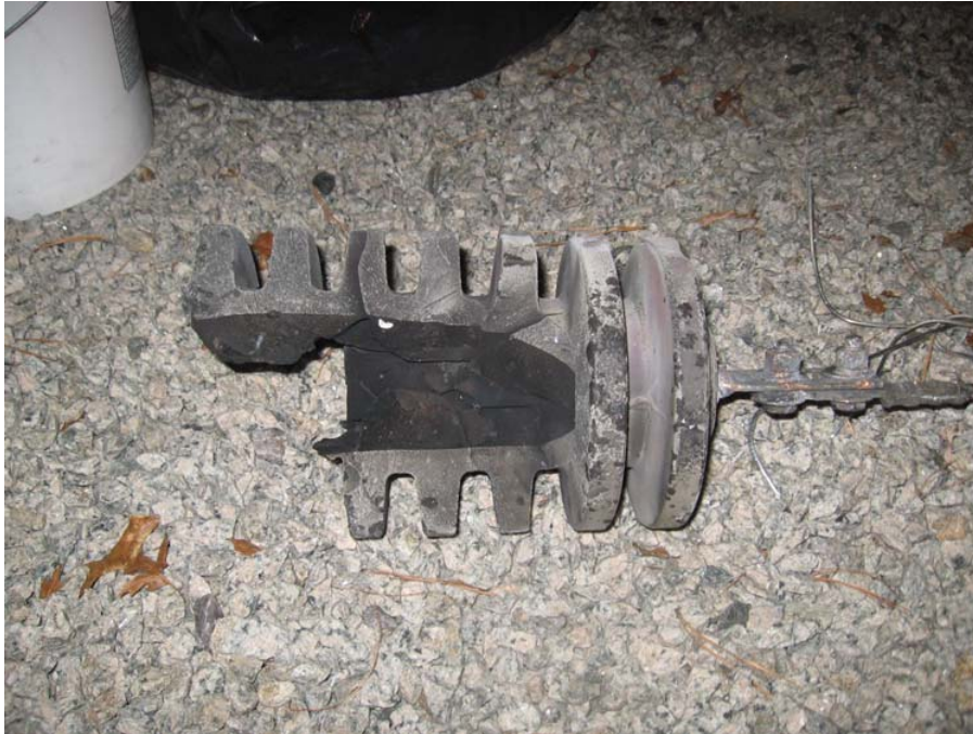
Figure 1 – Failed GE 34.5 kV Butyl Rubber Insulated PT
